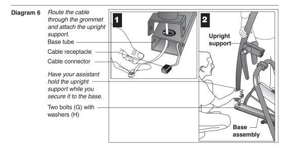
8. Position the upright support over the base. Diagram 6. Have your assistant move the upright support close to the front of the base assembly while you thread the cable through the grommet hole and out the front of the base tube (see inset #1). Make sure that the display console (on the upright support) faces the rear of the unit (see inset #2).
